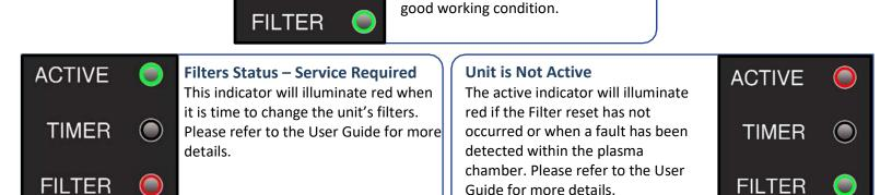
Changing the unit filters every 30 days is critical. Once the filter status indicator illuminates red, you have 15 days before the unit shuts off. Please refer to the User Guide for more detail.
